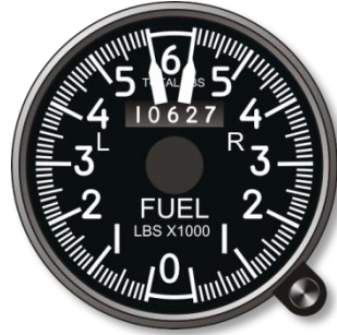
Figure 58. Fuel Quantity Indicator
